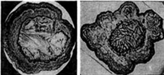
Fig. 2. Artificial agate structures on the base of KNO<sub>3</sub> composition
