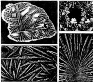
Fig. 1. Different dendrite structures of KNO<sub>3</sub> decorative coating
